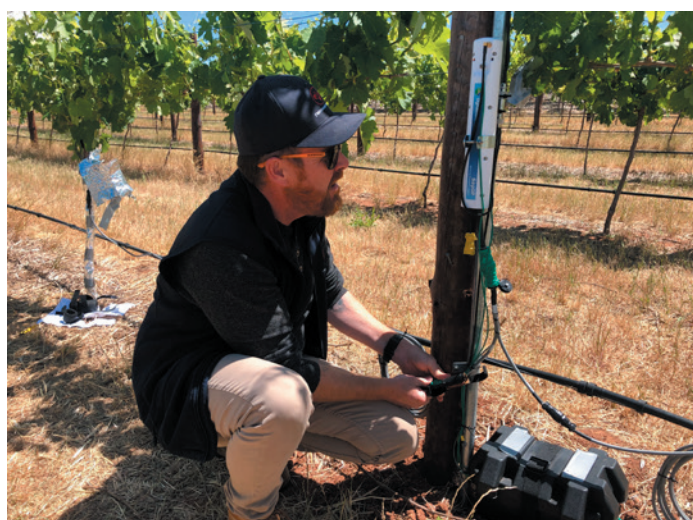
Two Hands viticultural manager Travis Coombe checks a sap flow sensor (left) and the relay that sends the data collected by the sensors to a web interface (right).
