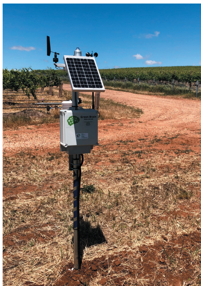
The weather station in Two Hands’ Seppeltsfield vineyard, which assists in relaying the data collected by the sap flow sensors to a web interface where it can be analysed.
